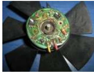
Removing the fins from the housing, the controller is revealed
