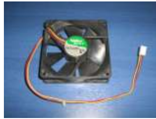
PC fans use BLDCs for their silent operation and reliability
